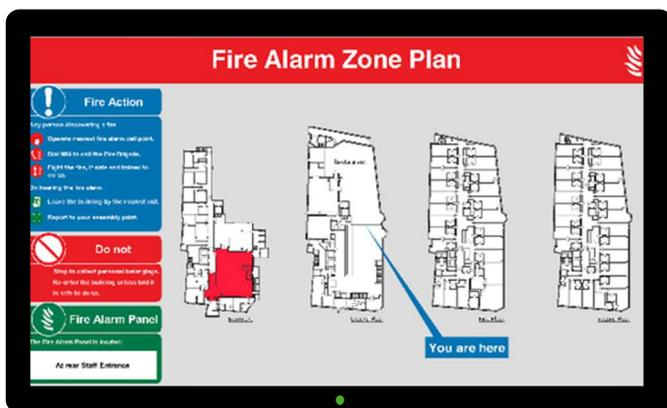
On activation of a fire alarm in your premises, dynamicZM will automatically display the zones (areas) where the fire has been reported and highlights the zone of origin. Once the fire alarm has been cleared and the system reset, dynamicZM will return to the scheduled media display automatically.
