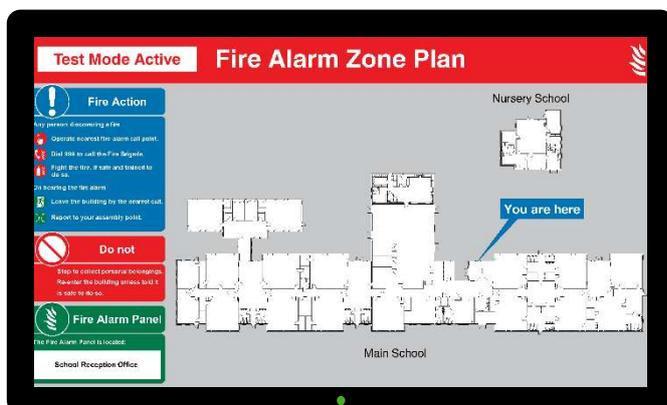
dynamicZM has a test facility to check that the building plan is correct and ready for activation by the fire alarm system. Activating the test mode **does not** activate the fire alarm control panel or sounders in your building. Switch the test switch only once. When activated, the test mode will self-reset after approximately 60 seconds.
