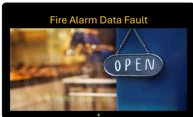
If dynamicZM can no longer receive a signal from the fire alarm system a Fire Alarm Data Fault notification will appear at the top of the screen. The fire alarm control panel will also report a fault condition. Media will continue to play and the notification will turn off automatically when the fault has been rectified.
