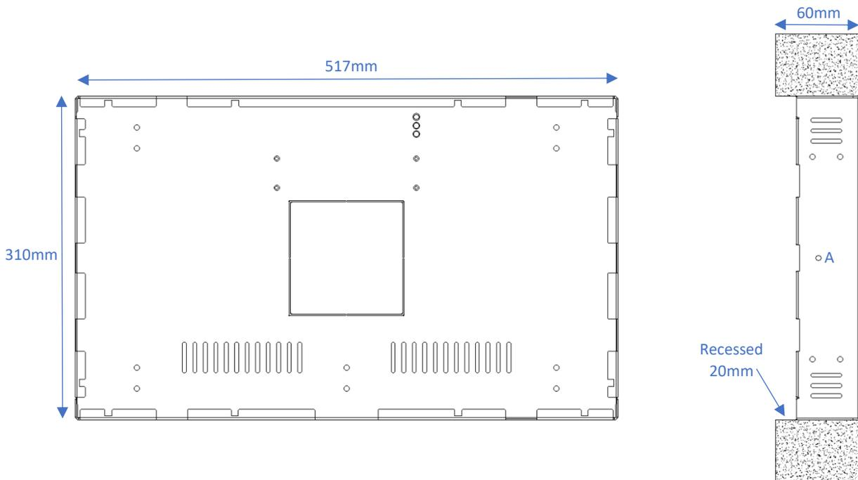
Note 1 - The backbox should be recessed **20mm** from the wall face, to allow the dynamicZM to be flush against the installation surface when fitted. See Fig. 1. and Fig. 2.
