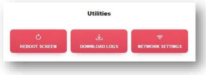
**6.5.1 Network Settings** – this opens your PC network settings for you to connect to the dynamicZM via wi-fi. You must be connected to the dynamicZM to carry out all other operations within this engineers tool.
