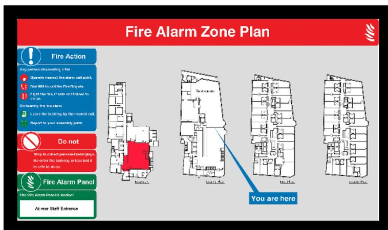
In a fire condition, the dynamicZM displays the zone plan layout and indicates the zone(s) in alarm. The first zone to be activated is shown with a flashing outline as an indicator of the zone of origin of the fire alarm. Further zones are shown solid indicating the subsequent spread of the fire alarm activations.
